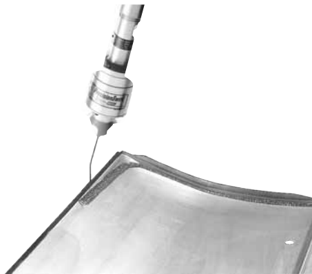
Width and thickness of swirl are controlled with flow rate, analog signal, or application speed.
