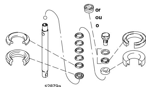
Soak leather packings in SAE 30W oil for 1 hour before assembly.
