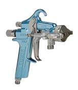
\*Binks Mach 1 PC Gun is a two component HVLP spray gun with external catalyst injection. Catalyst is injected through the air cap with atomizing air.
